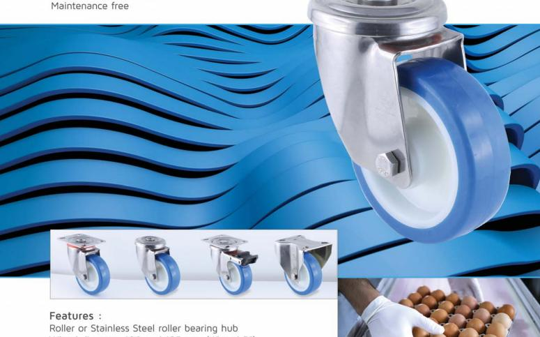
Wheel diameter 100 and 125 mm (4" and 5") Wheels load capacity 180 to 210 Kg (396 to 462 Lbs) Castors load capacity 180 to 210 Kg (396 to 462 Lbs) High pressure washable Temperature resistant -40°C +90°C (-40°F +194°F)
